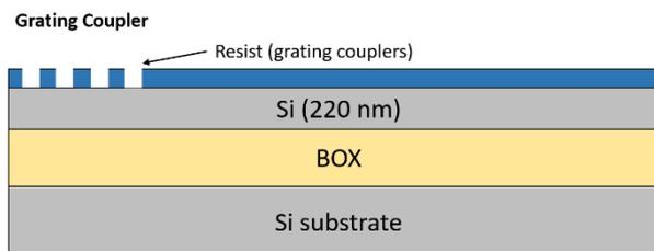
3. Shallow Si etch ( $70 \text{ nm} \pm 10 \text{ nm}$  etch depth)
