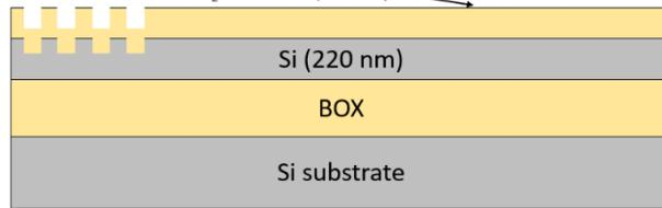
6. Resist patterning for Silicon Etch 2 (GDS layers 3 & 4) – 120 nm ± 10 nm etch
