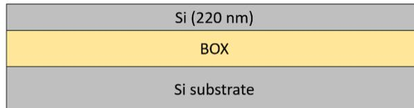
2. Resist patterning for Silicon Etch 1 (GDS layer 6) –  $70 \text{ nm} \pm 10 \text{ nm}$  etch
