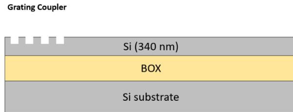
5. Resist patterning for Silicon Etch 2 (GDS layers 3 & 4) – 340 nm etch to BOX
