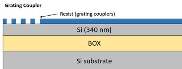
3. Shallow Si etch ( $195\text{ nm} \pm 10\text{ nm}$  etch depth)
