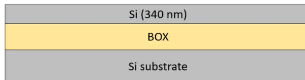
2. E-beam resist patterning for Silicon Etch 5 (GDS layer 60) –  $195 \text{ nm} \pm 10 \text{ nm}$  etch
