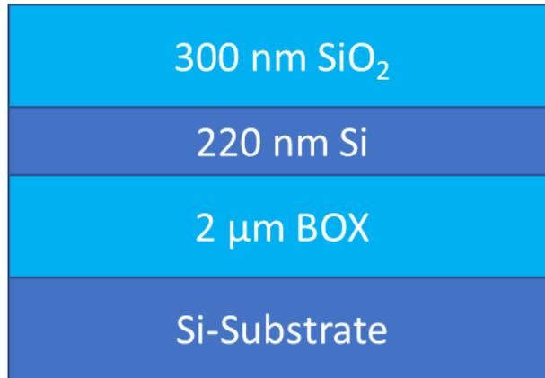
*Figure 1 Sample layer stack of 300 nm SiO<sub>2</sub> on 220nm Si on 2μm BOX on Si substrate*
