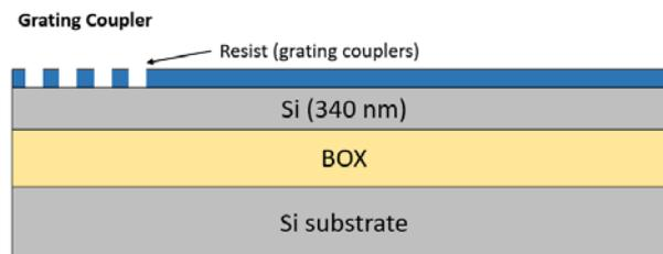
3. Shallow Si etch ( $140 \text{ nm} \pm 10 \text{ nm}$  etch depth)
