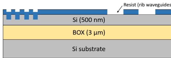
6. Intermediate Si etch (300 nm ± 20 nm etch depth)
