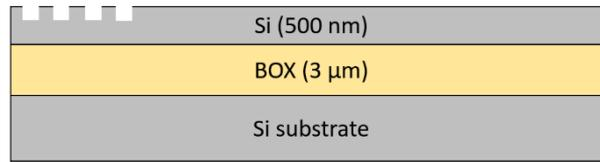
5. Resist patterning for Silicon Etch 2 (GDS layers 3 & 4) – 300 nm ± 20 nm etch
