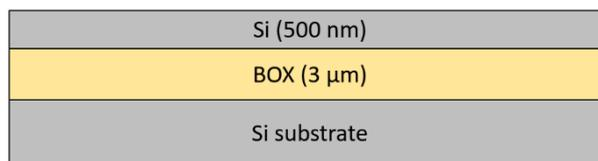
2. Resist patterning for Silicon Etch 1 (GDS layer 6) –  $160 \text{ nm} \pm 15 \text{ nm}$  etch
