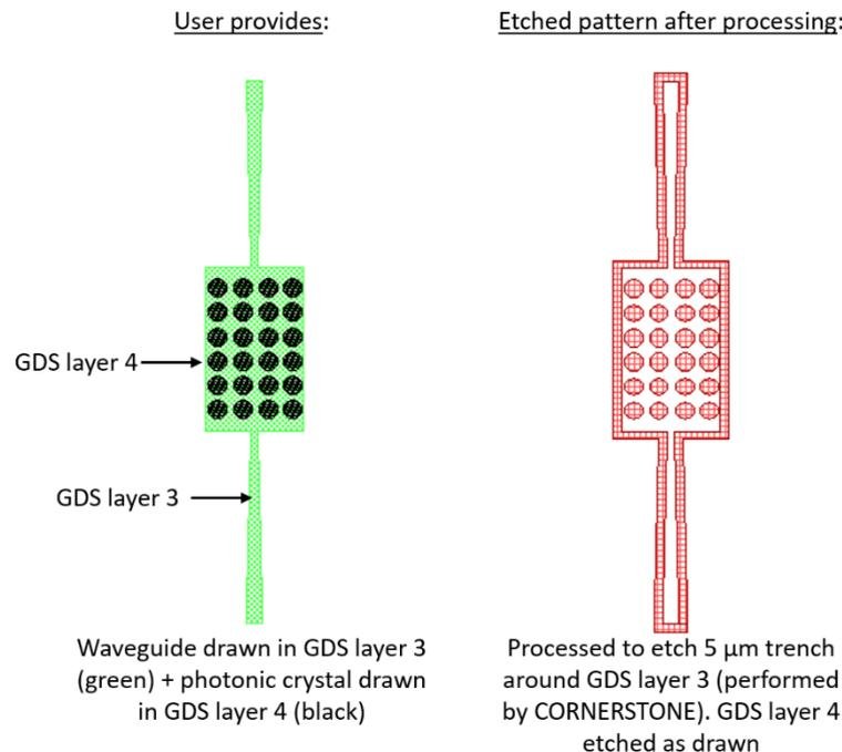
Figure 3 – Example photonic crystal structure using GDS Layers 3 & 4.
