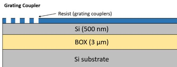
3. Shallow Si etch ( $160 \text{ nm} \pm 15 \text{ nm}$  etch depth)
