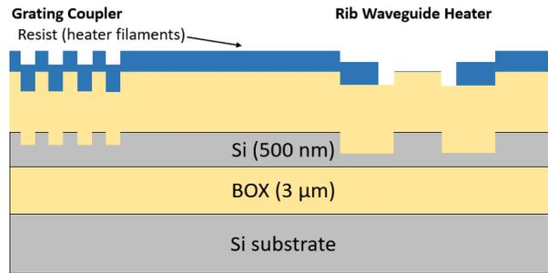
10. Heater filament deposition
