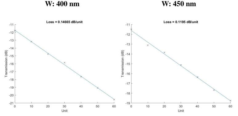
Transmission includes the measurement system loss, grating coupler loss and waveguide loss, as well as the measured device loss
