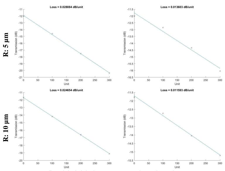
Transmission includes the measurement system loss, grating coupler loss and waveguide loss, as well as the measured device loss
