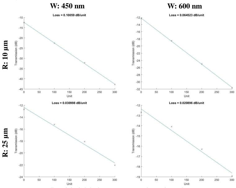
Transmission includes the measurement system loss, grating coupler loss and waveguide loss, as well as the measured device loss
