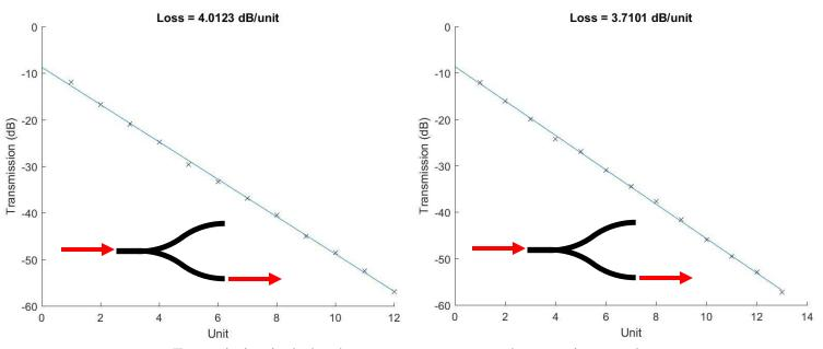
Transmission includes the measurement system loss, grating coupler loss and waveguide loss, as well as the measured device loss
